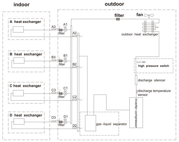
A1:A-unit electronic expansion valve B1:B-unit electronic expansion valve C1:C-unit electronic expansion valve D1:D-unit electronic expansion valve A2:A-unit gas pipe temperature sensor C2:C-unit gas pipe temperature sensor A3:A-unit liquid pipe temperature sensor C3:C-unit liquid pipe temperature sensor D3:D-unit liquid pipe temperature sensor D3:D-unit liquid pipe temperature sensor
