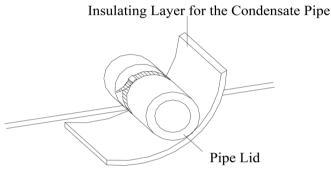
Fig.13 Thermal Insulation of the Condensate Pipe
